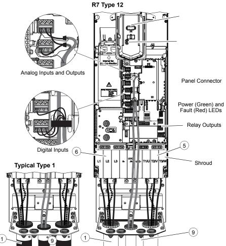
Note: UDC+ and UDC- terminals are used for external brake chopper units.
