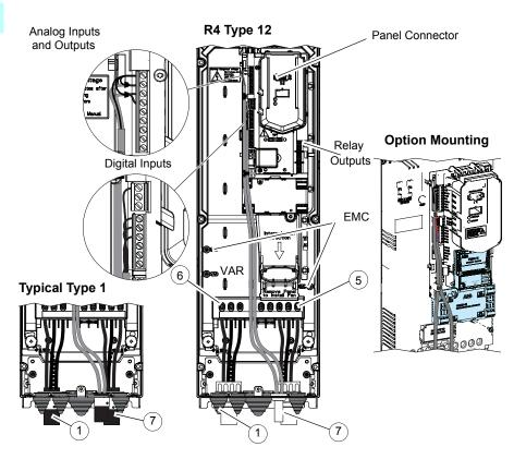
Note: UDC+ and UDC- terminals are used for external brake chopper units.
